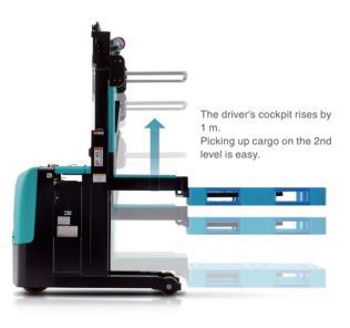
This compact picker can increase the working area as picking face up to the 2nd level. It is possible to utilize the 2nd level, to double the storage capacity by flat picking sites or to change the capacity of products which vary with seasons. The design accommodates various conditions on site according to the use.
